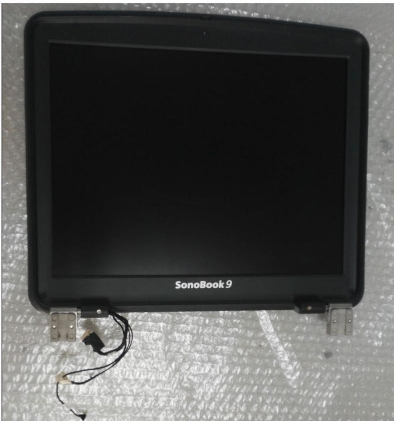
**⚠️ NOTE:** While take out the LCD MODULE , carefully disconnect the LCD cable, avoid any damage for the cable.
