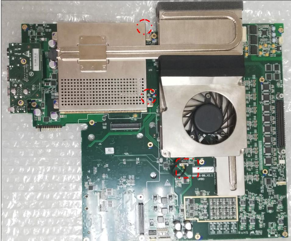
2) Remove the 6 screws on the back of the MAIN BOARD.
