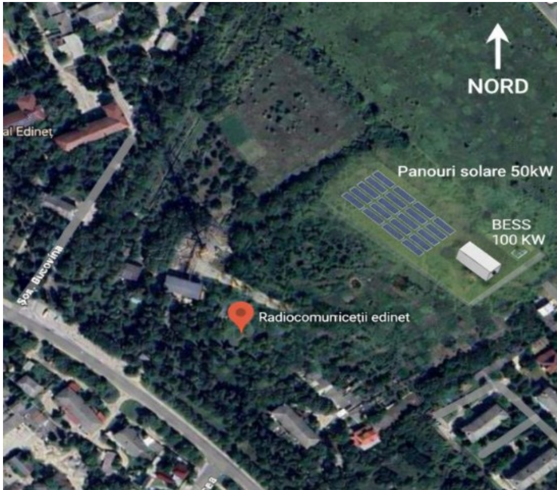
Fig. 2. Layout of the Photovoltaic Panels Arrangement
