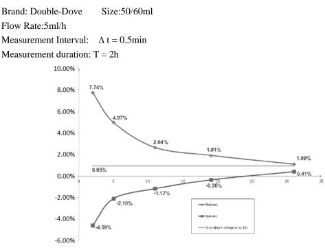
Graph 4 Trumpet curve: Percentage variation Ep against observation window duration P (min) and the overall mean percentage error A plotted from data gathered during the second hour of the test period
