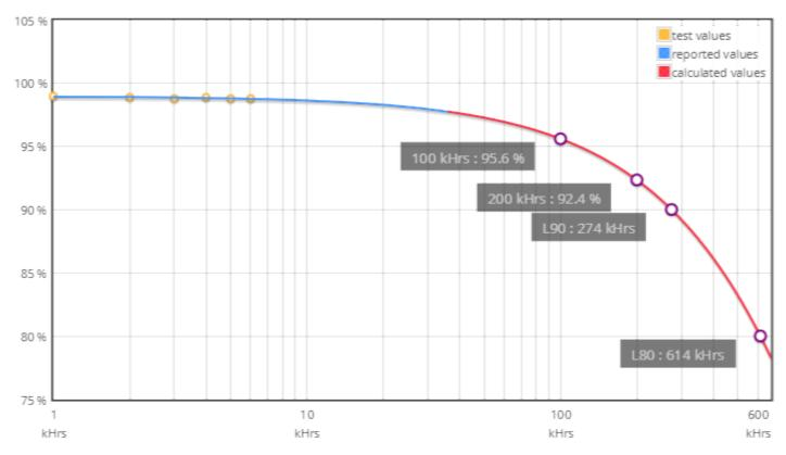
LxB50 results according to LM-80 and TM-21 procedures and norms. LxBy results derived from LxB50 according to IEC 62717 Annex C.
