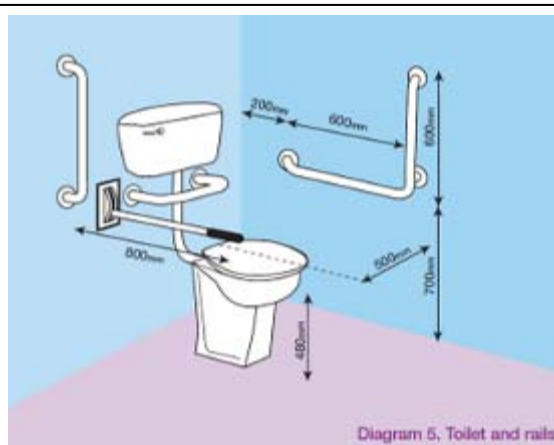
Typical location and size of stainless steel bars around the toilet.
