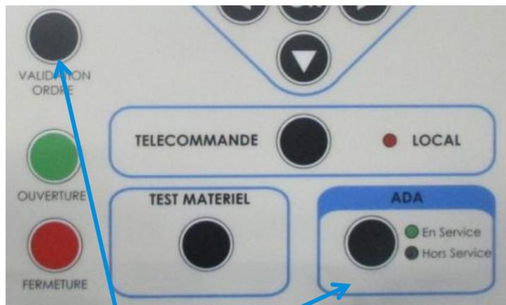
To activate the ASF function, press the “ASF” and "COMMAND VALIDATION" buttons at the same time. After activation, the green "ASF on" indicator light is illuminated
