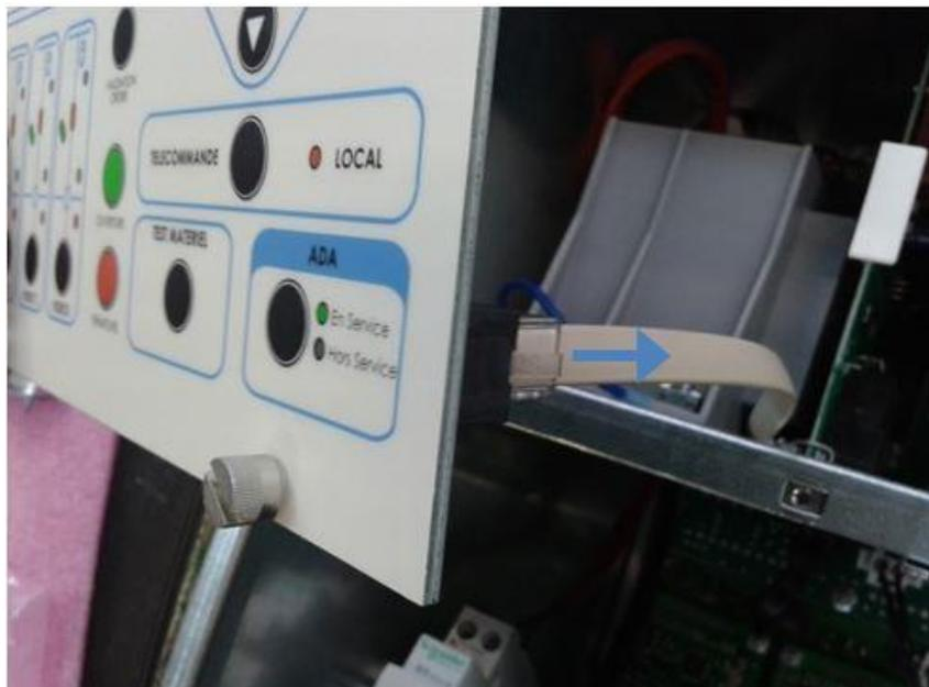
You must remove the locking clips to remove the charger and converter boards.
