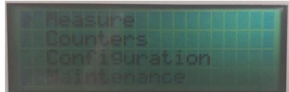
Position the arrow opposite a tab and press the OK button to access it. To leave the tab, press the LEFT button. The arrow is moved using the UP and DOWN buttons.
