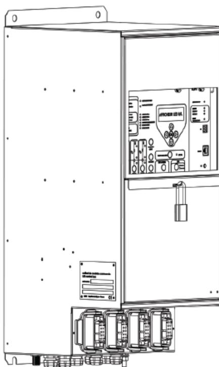
**Level 1: Operation:** access for operating personnel. Only the user interface (UI) is accessible. The upper part is locked using two seals.
