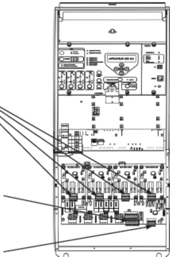
Note: For the e-RTU2020-2S version only two "HARTING" type connectors and two current acquisition modules are installed on the product.
