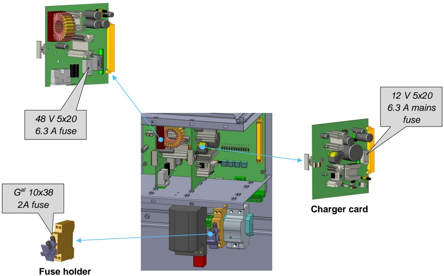
Should the equipment malfunction (to identify the problem see §5.1), it may be necessary to replace a cabinet component (electronic circuit board, battery, cable, etc.).
