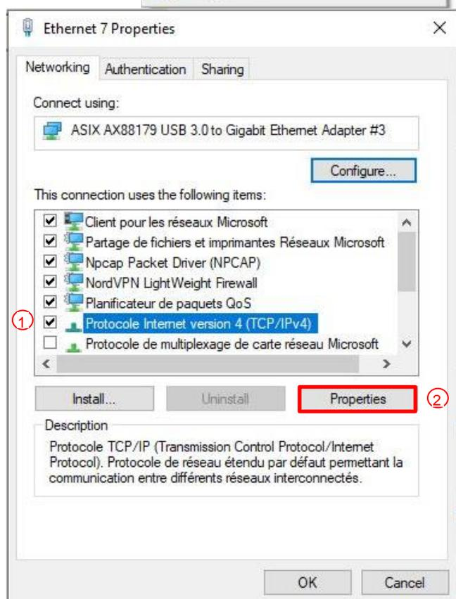
① Select “Internet Protocol (TCP/IP)” or “Internet Protocol version 4 (TCP/IPv4)” (without deselecting the check box)
