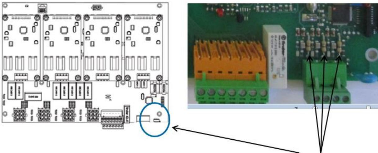
To do this, you need to use suitable wire cutters to cut away the 3 standard resistors at the bottom right of the wiring board. Therefore, the calibration method is identical to that described above and presented in §3.2.
