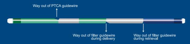
Delivery sheath provides gradient hardness. The softer diatal segment ensures outstanding kink resistance.
