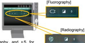
\*Density can be adjusted ±3 for Fluorography, and ±5 for Radiography.
