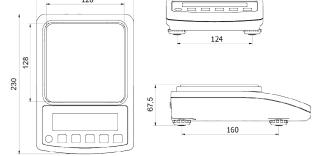
BWLC-TB balances are designed for fast and precise determination of mass in
