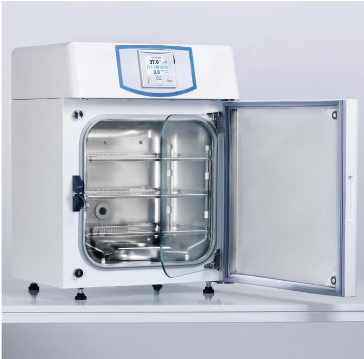
The newest generation of CO<sub>2</sub> incubators aims at constant and repeatable conditions for procedures of cells and tissues growth and other cultivation processes. The system of direct heating eliminates the necessity of a fan use and consequently it also eliminates the risks of vibrations and cross contamination. The infrared sensor without any variations provides maximal reliability and precision of measuring in the course of the whole process.
