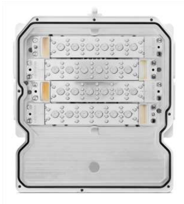
Figure 29: Open OCU Showing the Channel Filters
