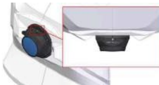
Figura 290. Adaptor UWF rotit corect.
