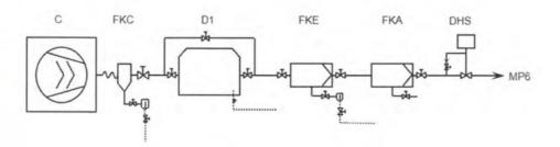
C: KAESER oil cooled screw compressor FKC: liquid separator D1: KAESER refrigeration dryer FKE: KAESER micro filter KE FKA: KAESER activated carbon filter KA
