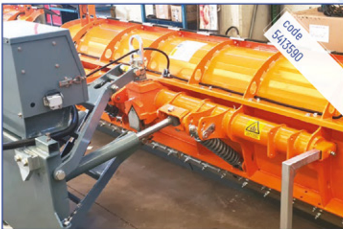
Anti-shock system through pressurized springs
