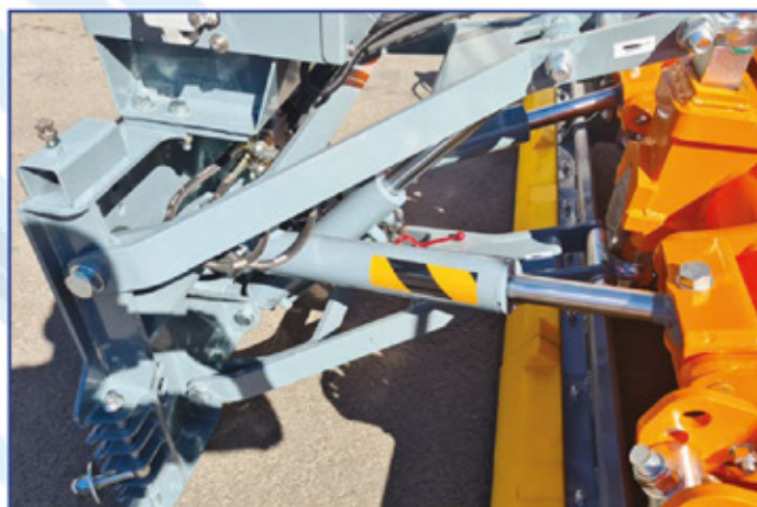
Lifting system by double-acting cylinder and orientation by n.2 single-acting hydraulic cylinders, equipped with anti-shock valve
