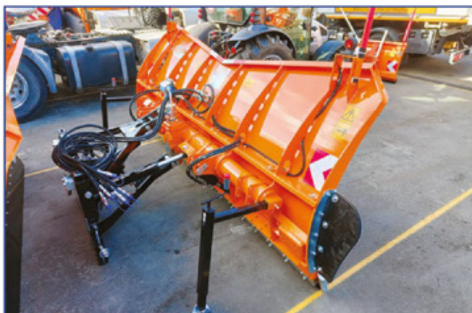
"V"-shaped upper extension - H.1100 mm / H.1400 mm
