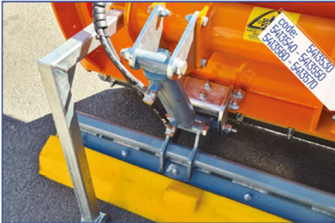
Hydraulic adjustment 2nd Vulkollan cutting edge
