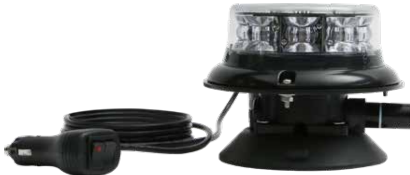
3-3751-S suction mounted ELP beacon with 3-1000 lead and double switch fused plug
