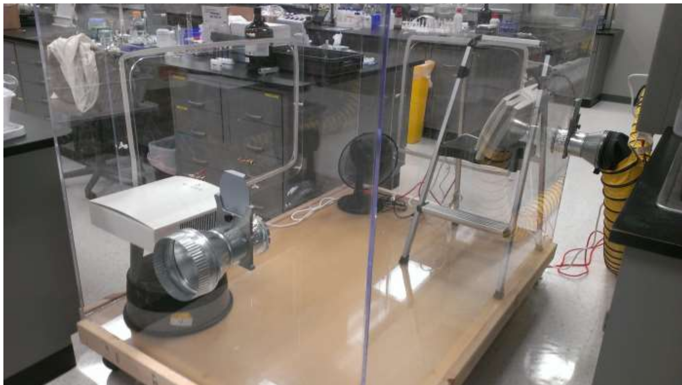
Figure 3: Plexiglas chamber for formaldehyde removal testing.
