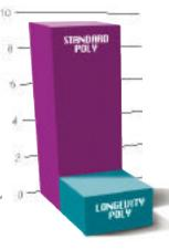
Effect of Crosslinking Wear Rate (mg/million cycles) of Longevity polyethylene and standar
