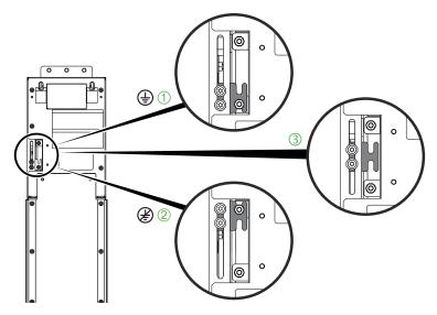
**NOTE:** Do not operate the module with the EMC filter bracket removed or with the EMC filter bracket in the middle position ③.
