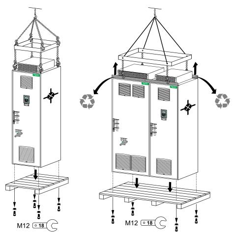
Mount the handling lugs, which are provided in a separate packaging.
