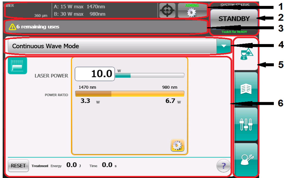
Figure 3: Subdivision of the operating interface
