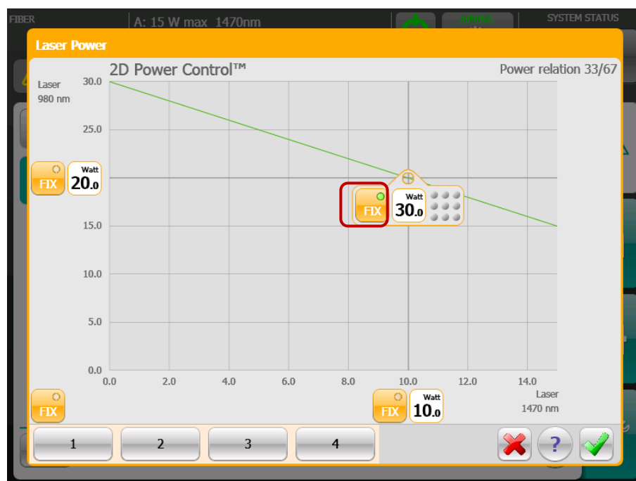
Figure 18: Setting output with constant total laser power output
