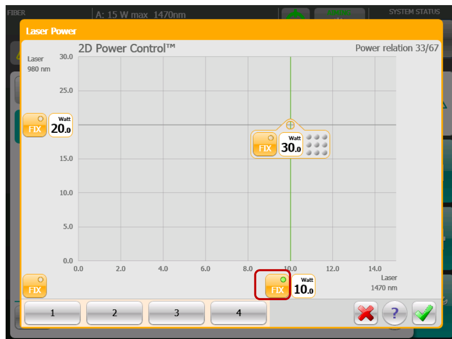
Figure 20: Fixing the power for the wavelength 1470 nm on the horizontal
