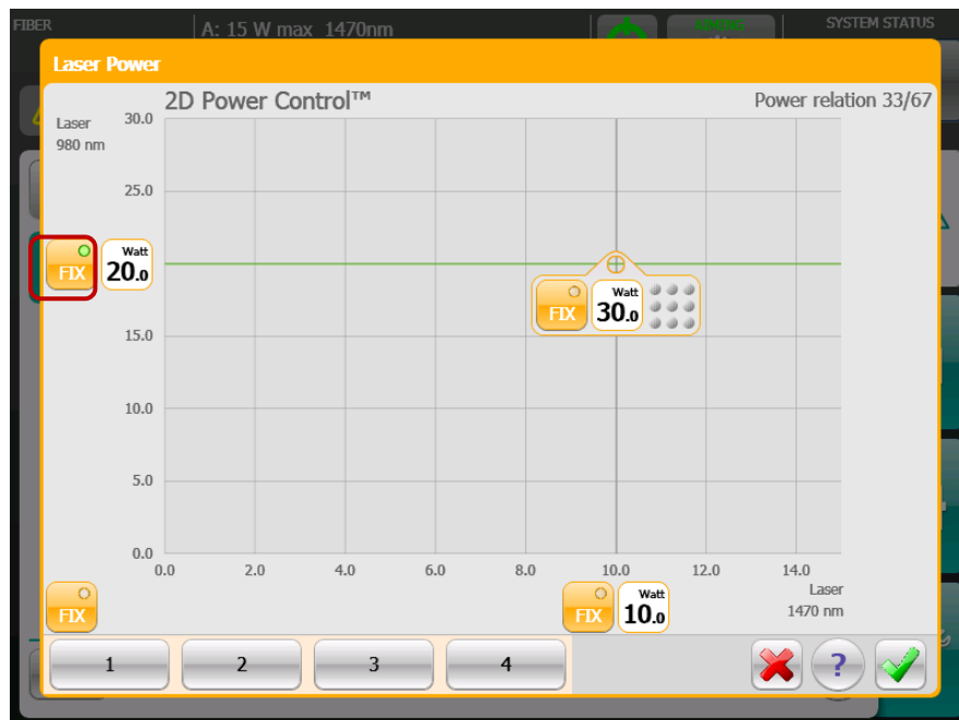
Figure 21: Fixing the power for the wavelength 980nm/1064nm on the vertical axis
