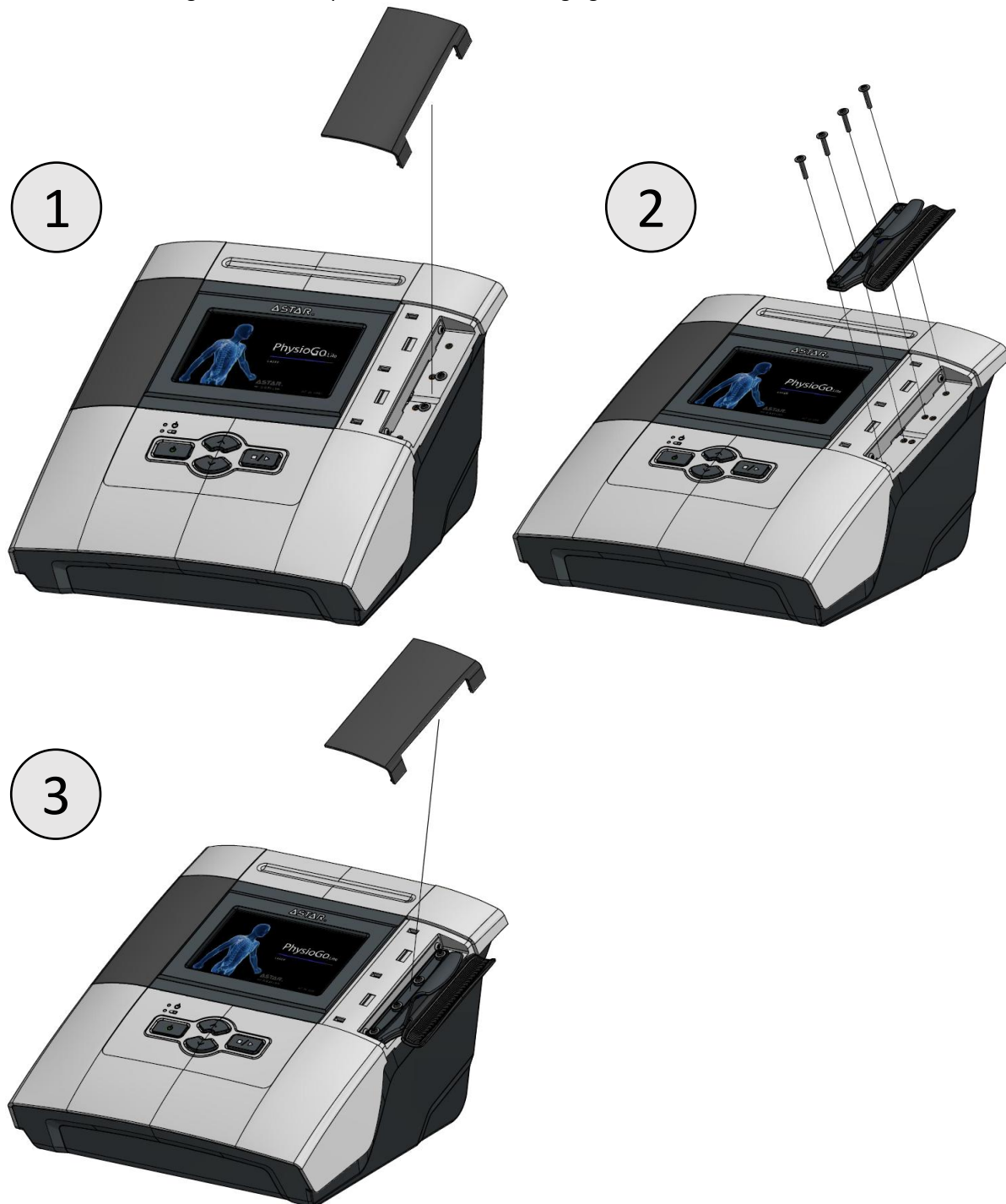
Figure 6-1 Method of mounting the point applicator holder
