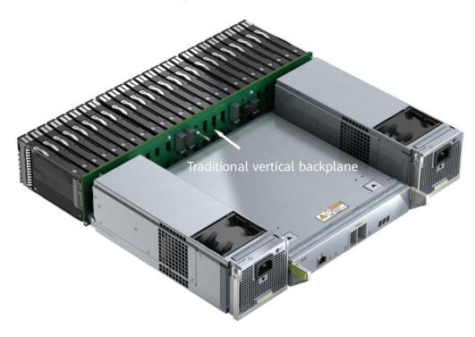
Figure 3-18 Front view of the window areas on the vertical backplane
