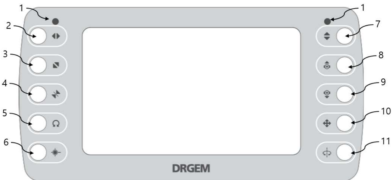
Tube Head Control Button (Option: Motorized Tube Rotation - TS_FM6, TS_FC6)
