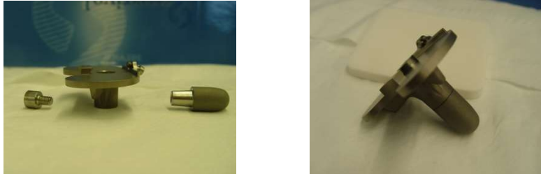
(Image 2 & 3: preassembly of tibial tray components)
