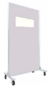
Lead glass shield (partial shield) N-XR-g-3 180(L)x90(W)cm with 20(L)x30(W)cm window size Protection: 1.65 mmPb. Lead glass thickness: 8 mm Lead plate thickness: 1.5 mm
