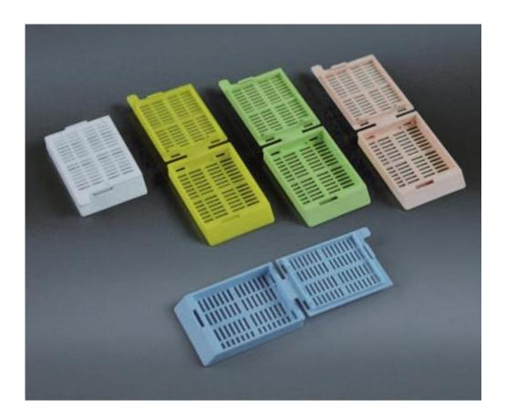
Rectangular grid, in acetal resin (POM), with lid provided with two safety locking points, removable. Writing surface. They resist to decalcifying solutions, to solvents and ultrasounds techniques. Compatible with most of automatic autoloader printers (Leica IP C ecc.). Dimensions 40 x 28 x 6 mm. Printing front side at 45°.
