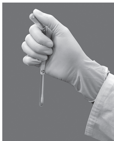
Break the red „snap“ valve by bending to a 45° angle.
