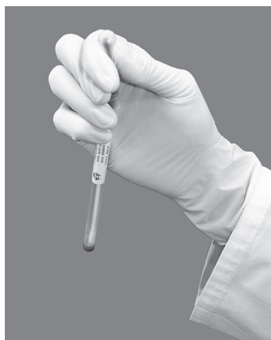
Gently squeeze cap until all fluid moistens the lyophilized pellet in the bottom of the tube.
