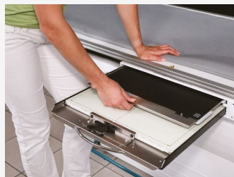
Cassette tray / Bucky with exchangable grid
