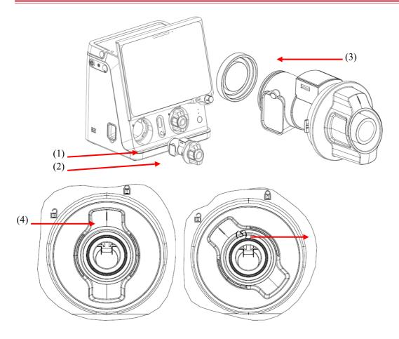
Expiratory valve component Expiratory valve locked status
