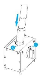
Figure 14: Using SharpAdjust to fine-tune the handpiece optics
