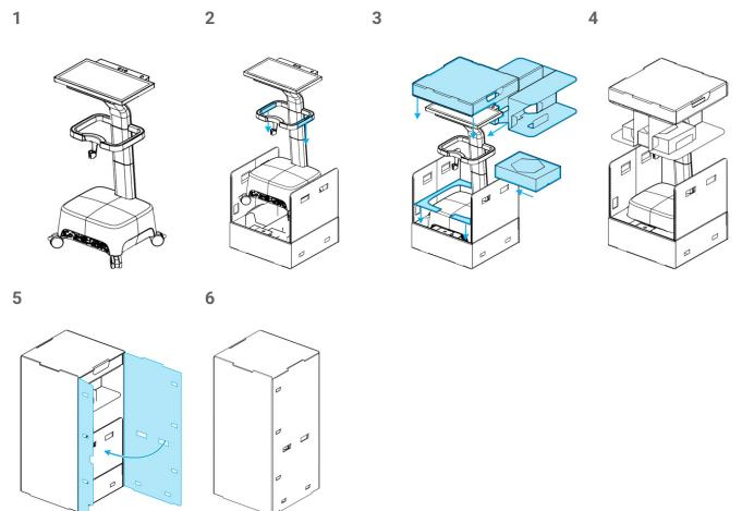
Figure 16: Steps for packing the scanner - Model 001 (cart)
