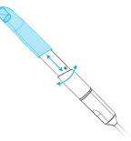
Figure 7: Assembling and disassembling the handpiece sleeve
