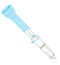
Figure 10: Using the integrity-check sleeve
