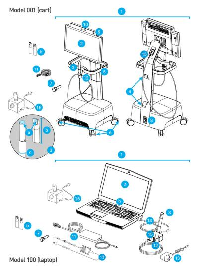
Figure 4: Identification of the scanner parts
