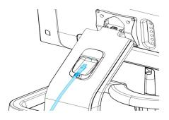
Figure 5: Plugging the handpiece – Model 001 (cart)
