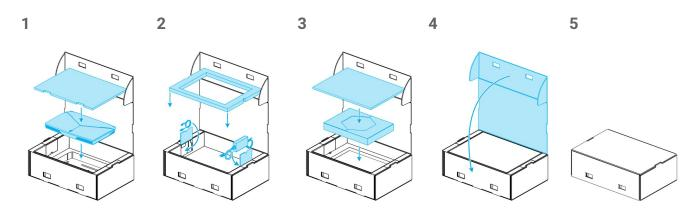
Figure 17: Steps for packing the scanner - Model 100 (laptop)
