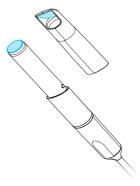
Figure 8: Cleaning the optics of handpiece and sleeve
