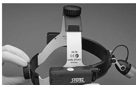
4. Set the orientation of the LED light and the diameter of the illuminated field using the rotating ring on the lamp head.
