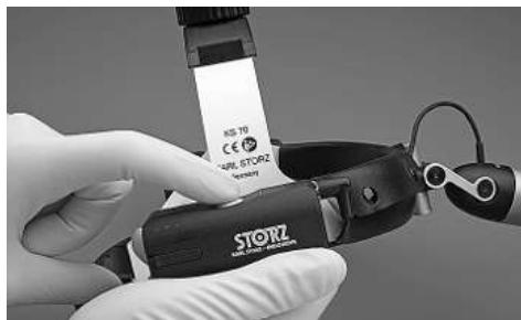
2. Remove the batteries from the control unit and from the battery box.
