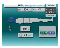
After the user confirms no air is present in the system, it is still possible conditions are not sufficient for the injection to start. If "Air Check" has been pressed, but the injection cannot be performed, a "Not Ready" state will be presented to the user. The "Not Ready" state appears as a blinking "Not Ready" in the upper right corner of the display.
