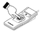
An injection can be started in the control room by pressing the Start button on the Switch Box or by pressing the Start button located on the Powerhead.
