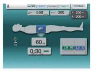
Input your date once, and from there the alpha? will calculate the injection rate automatically. Just selecting an anatomic region, the alpha? can calculate the contrast media volume required for your protocol.
