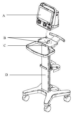
A. Main unit B. Positioning post C. Trolley unlocking button D. Trolley Align the main unit with the two positioning posts on the trolley and put it onto the trolley in place.
