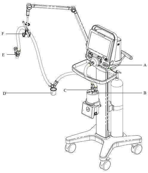
A. Inspiratory filterB. Humidifier inletC. Humidifier outletD. Inspiratory water trapE. Y piece (connect with the O2 therapy mask)F. Support arm hook
