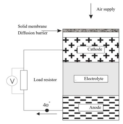
At the cathode oxygen is reduced to hydroxyl ions according to the equation:
