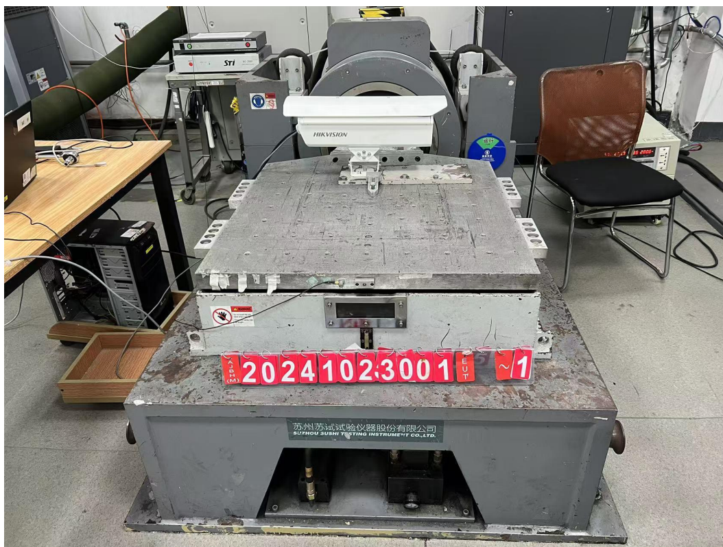
EUT-1 Y-axis layouts photo Random Vibration Test
