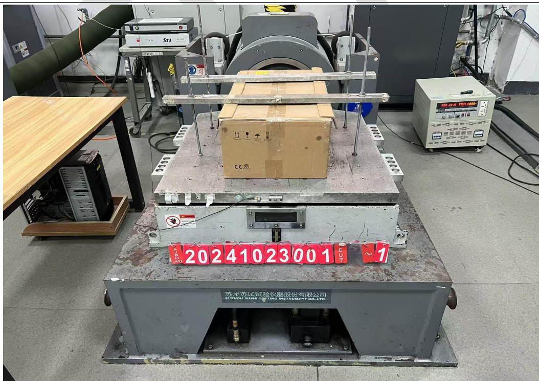
EUT-1 Y-axis layouts photo Random vibration Test(packaging)
