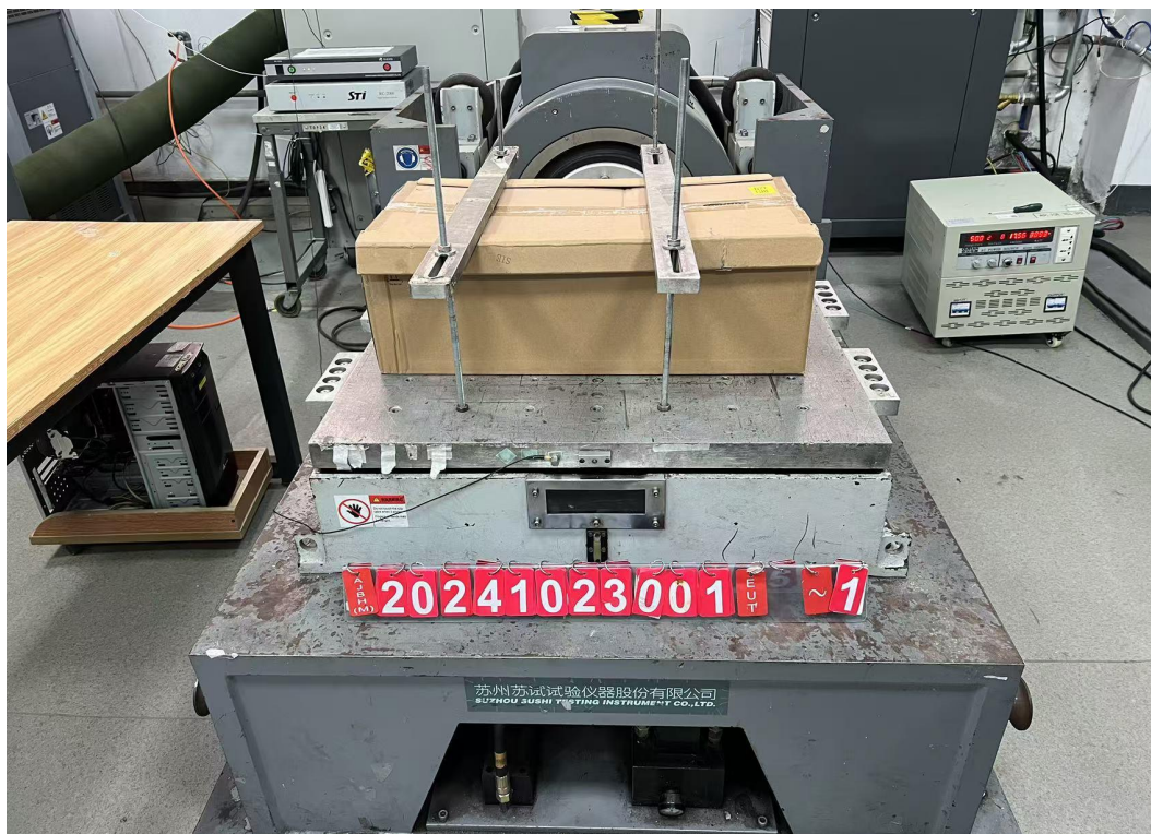
EUT-1 X axis fixed photo Random vibration Test(packaging)
