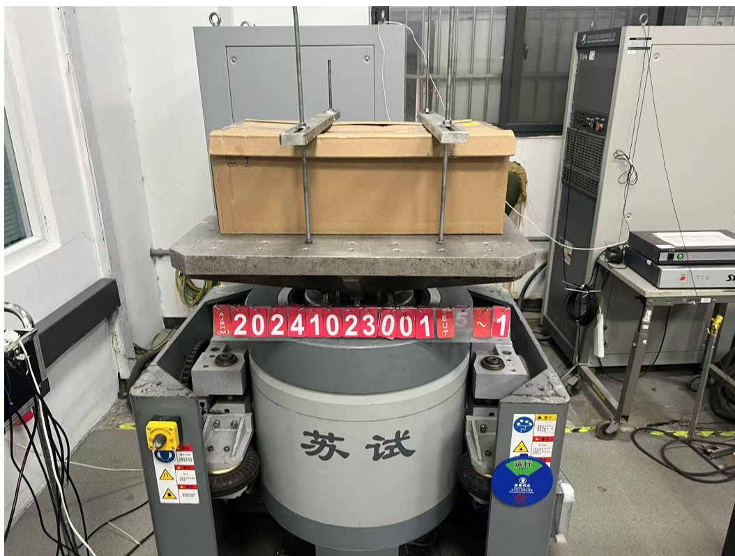
EUT-1 Z-axis layouts photo Random vibration Test(packaging)
