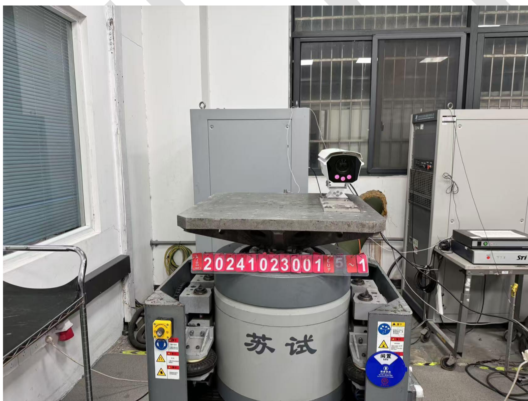
EUT-1 Z-axis layouts photo Random Vibration Test
