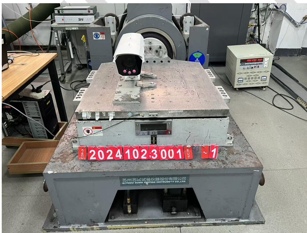
EUT-1 X-axis layouts photo Random Vibration Test
