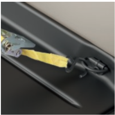
Sidewall tie-downs Transit's DIN/ISO compliant tie-down points are positioned just above the floor on the loadspace side walls. This makes it easier to secure loads, while keeping the floor clear of obstructions. (Standard)
