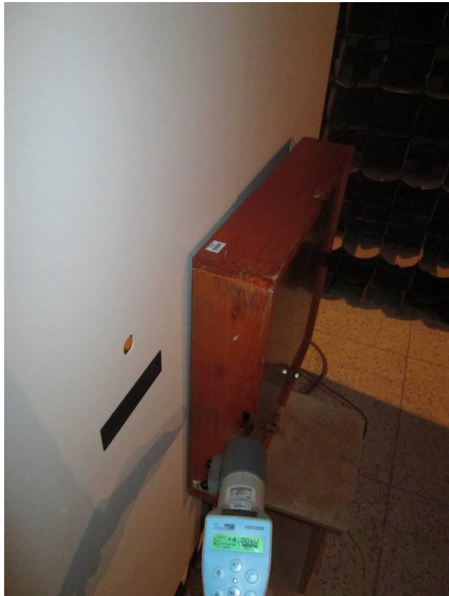
Indirect contact discharge Vertical plate
