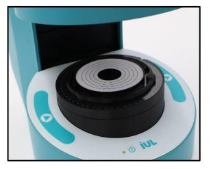
Push the Run button on the bottom right: **D** . The instrument will proceed to perform several image captures, and finally, an image of the calibration disk will appear on the Image Panel.
