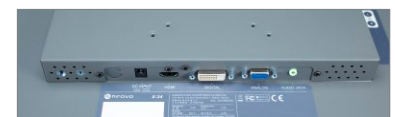
Multiple video inputs (HDMI, DVI, VGA, CVBS, S-Video) make possible effortless system integration
