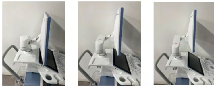
Figure 3-4 Adjusting the height of the monitor.
