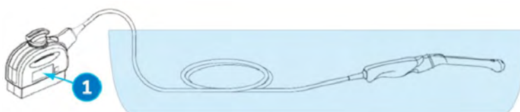
Figure 5-9 Probe Immersion Level for IC5-9-D
