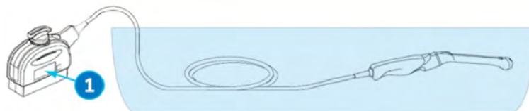
Figure 5-3 Probe Immersion Level for IC5-9-D
