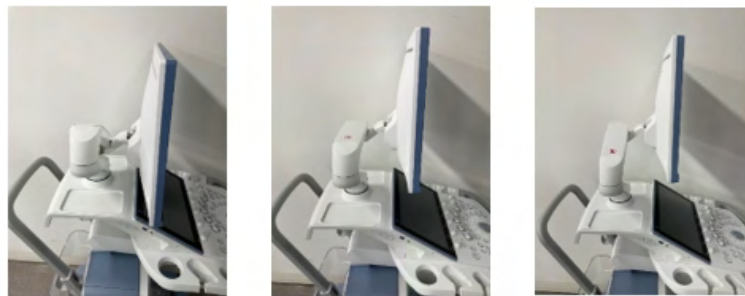
Figure 2-4 Adjusting the height of the monitor.
