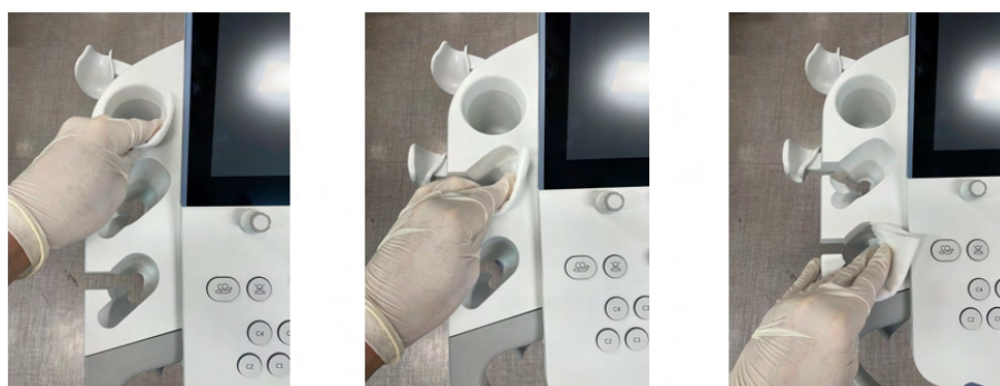
Figure 2-7 Cleaning and disinfection of the left Probe and Gel Holders. Repeat with shown procedure on the whole part
