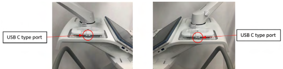
Figure 12-10 Install the charger on the left/right side
