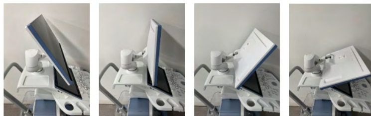
Figure 3-5 Adjusting the inclination of the monitor.
