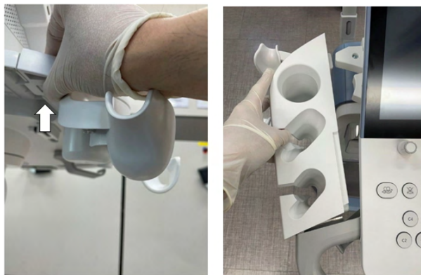
Figure 2-10 Removal of the left with Endocavity probe holder attached. For installation, just push them back into the user interface until you hear a “click” sound.
