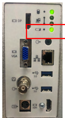
Figure 12-8 LED location of the battery
