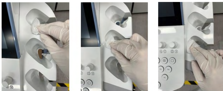
Figure 2-6 Cleaning and disinfection of the right Probe holder. Repeat with shown procedure on the whole part
