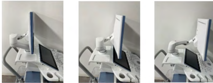
Figure 3-3 Adjusting the monitor back and forth.
