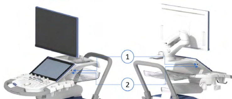
Figure 12-2 External I/O connectors
