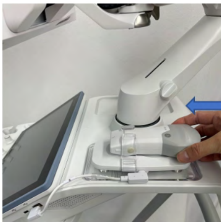
Figure 12-14 Install the charger on the right side
