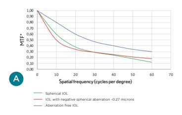
**A.** The IOLs are decentered 0.5 mm. Induction of asymmetrical HOAs degraded the performances of the spherical IOL and the one inducing negative spherical aberration, causing the MTF curves to droop and separate.
