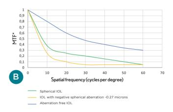
**B.** The IOLs are decentered 1.0 mm, further degrading performance of the spherical IOL and the one inducing negative spherical aberration IOL but not the aberration-free IOL.
