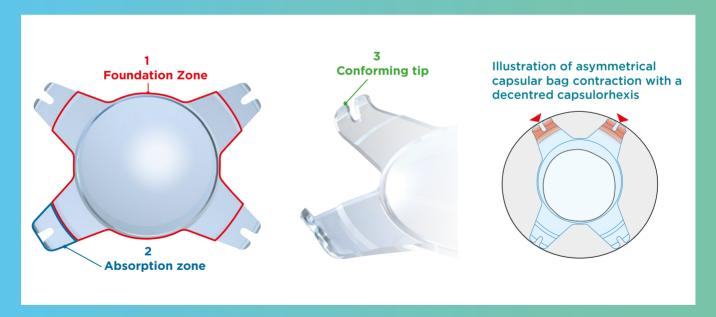
The Akreos® MICS IOL includes a foundation zone (1) formed by the optic and the base of the four haptics. This is the stable portion of the lens. It is surrounded by an absorption zone (2), which bends under the contraction forces of the capsular bag. The conforming tip (3) conforms to the curve of the periphery of the capsular bag and initiates the inflection of the absorption zone (2), which features an average 10° angulation.
