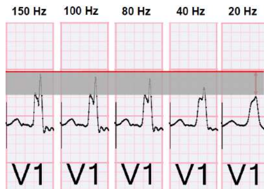
Lead V1 in Presence of RBBB at Different Low-Pass Filter Settings
