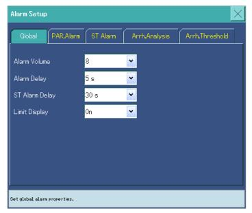
Figure 7.1 Alarm Setup Menu
