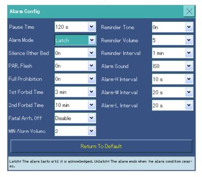
Figure 7.3 Alarm Configuration
