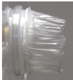
Fold back and slip elastic band over the outer ring of the port housing.
