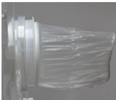
Install the smaller diameter elastic band of a new Sleeve over the inner ring of the port housing.
