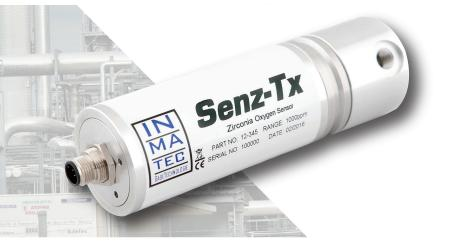
The Senz-Tx is a highly reliable and cost-effective two-wire, loop-powered transmitter with a linearized 4 to 20 mA output. It measures oxygen in 0-1000 ppm, 0-25% and 0-96% ranges. This compact transmitter uses proven zirconia sensor technology to accurately measure O2 in a variety of gases.
