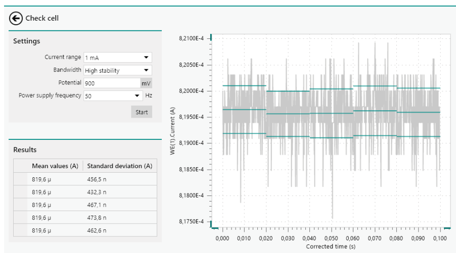
Figure 40 The Check cell tool can now be used to check the noise level
