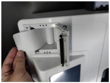
Figure 2-3-4 Installation diagram of print paper
