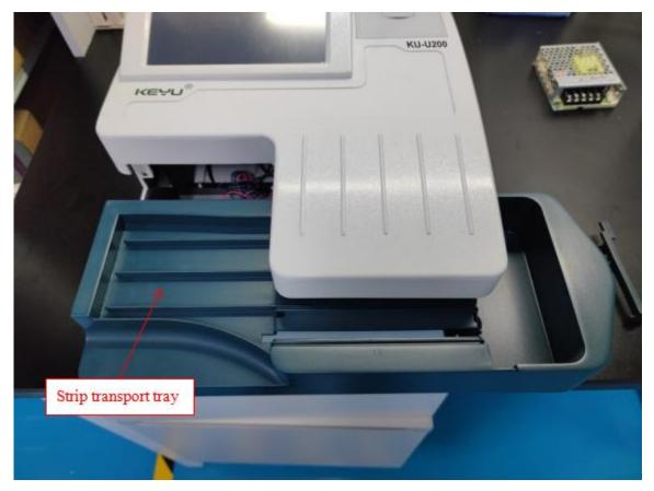
Figure 2-3-2 Installation diagram of strip transport tray
