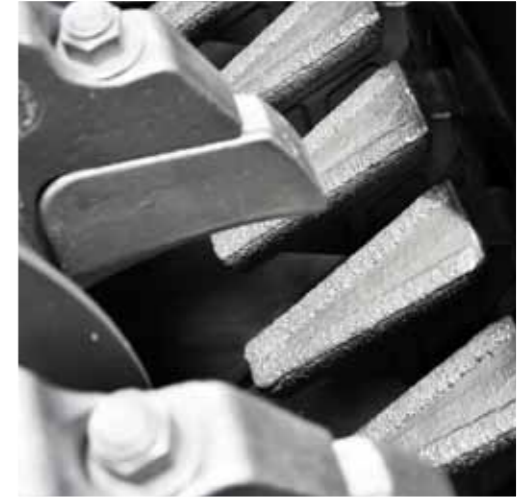
Counter knives. The grinding system tilting beam system with counterknives ensures long operations of the shredder allows removal of large, unbreakable materials - longer and troublefree operations of the machine. The standard electric reverse allows you to rotate the shaft in any direction without starting the combustion engine to remove blockages
