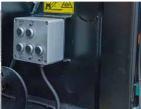
Rear control panel for safe and easy conveyors unfolding.
