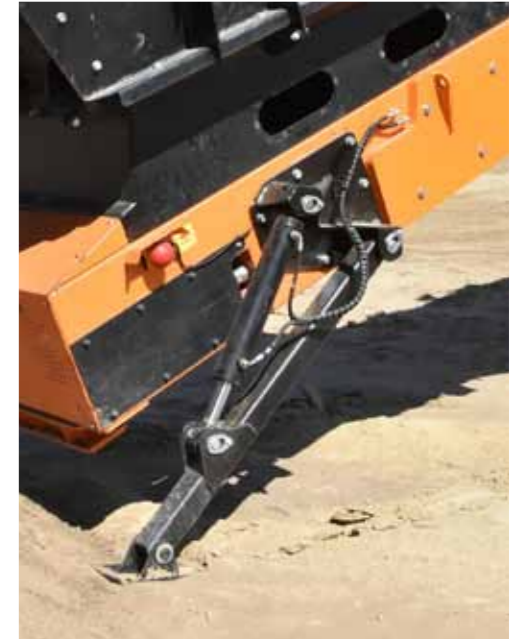
Hydraulic supporting legs (as an option) at the rear of the stockpiler
