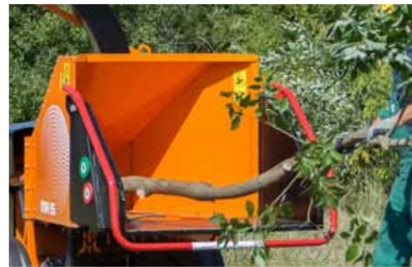
The branches are picked up automatically by means of hydraulically driven feed rollers.
