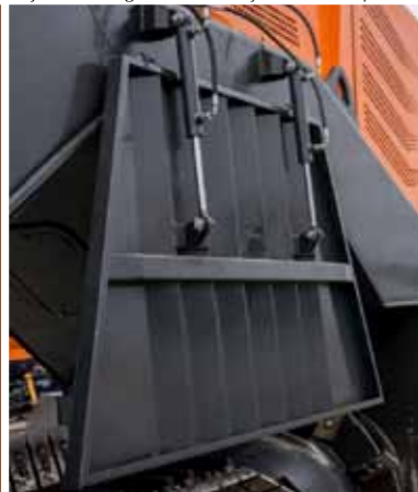
Adjustable tailgate limits the ejection of compost
