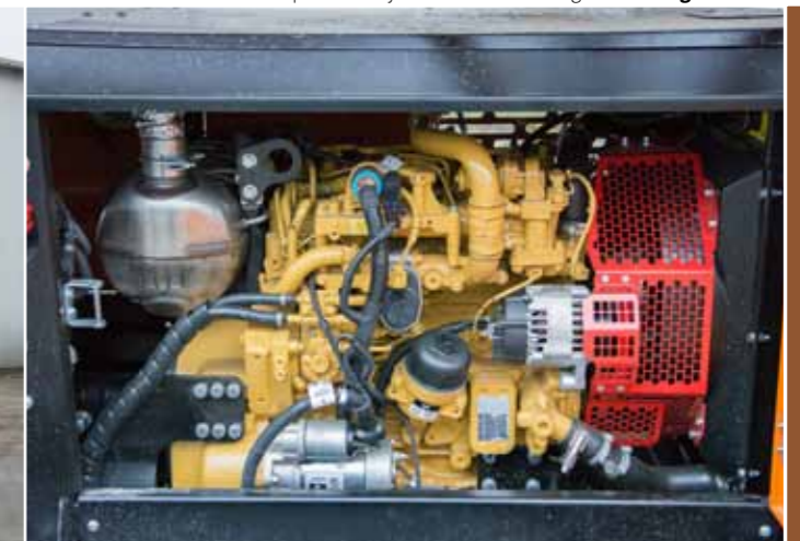
All functions of the device are powered by a 55.4 kW diesel engine CAT stage V
