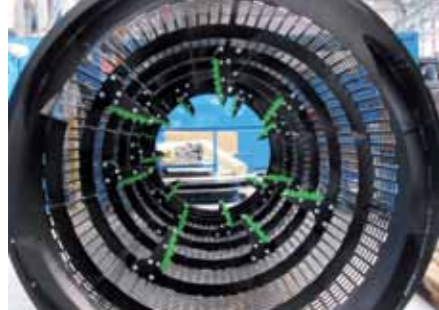
Screwed knives for ripping bags with waste*
