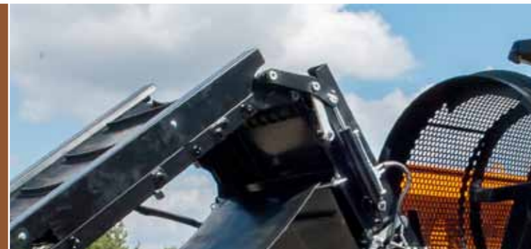
Rear conveyor folded by means of two hydraulic cylinders
