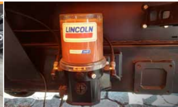
Central lubrication system ensures good greasing of the most important parts of the machine.
