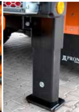
Hydraulic support legs ensures stability of machine
