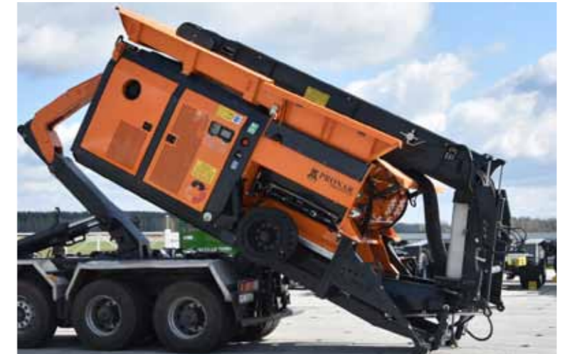
Hooklift standard. Machine designed with easy transport in mind on a three-axle truck thanks to low weight (~16 000 kg).
