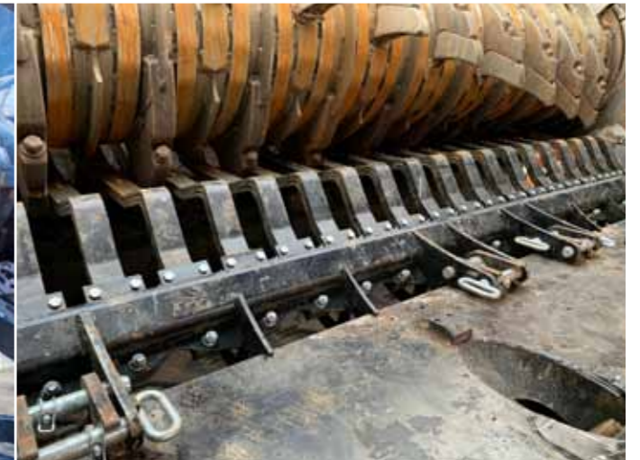
Steel bars for shredding more contaminated material and still getting proper fraction size.
