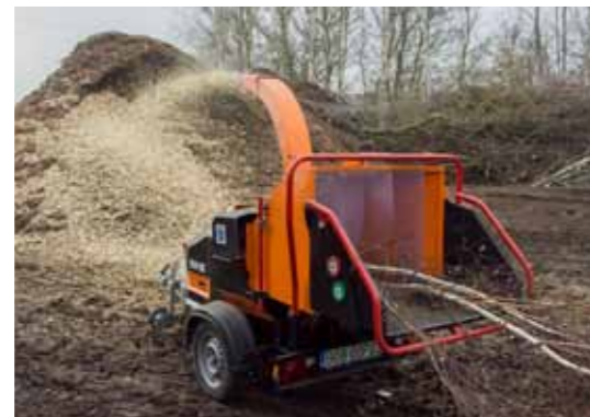
Loading ramp and safety bar.
