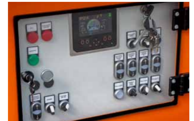
The functional control panel allows to monitor and set work parameters of the stockpiler
