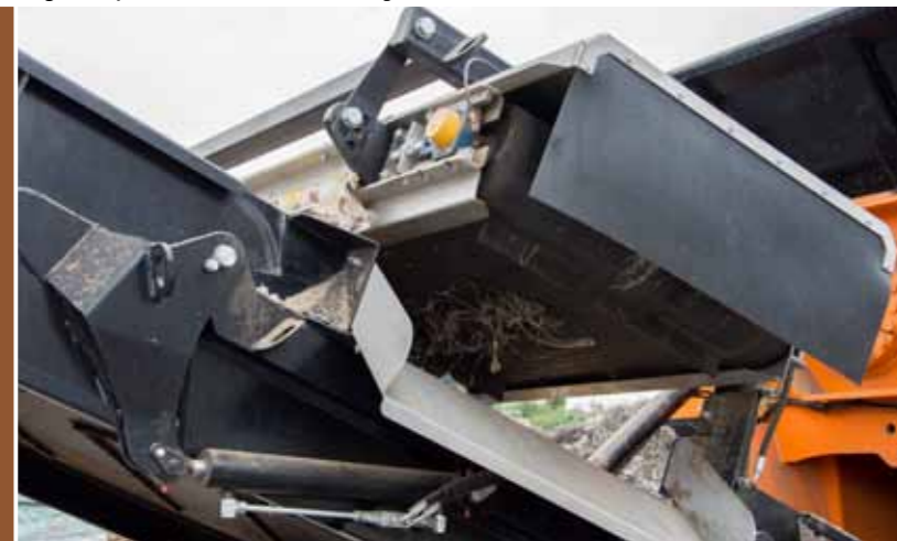
Magnetic separator for extraction of ferromagnetic materials.
