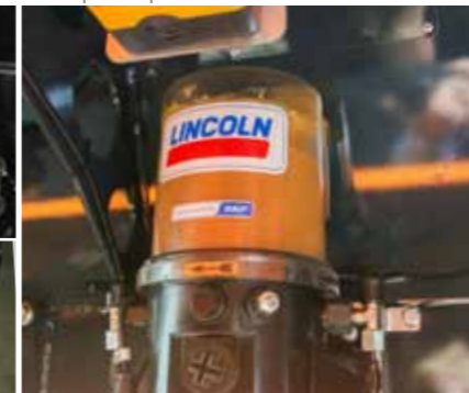
Central lubrication system ensures good greasing of most important parts of the machine
