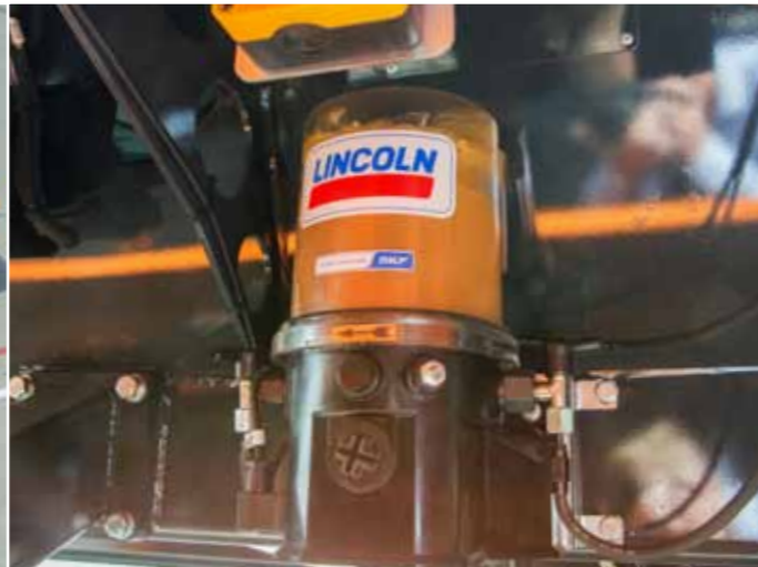
Central lubrication system. Makes sure that every point is properly lubricated.
