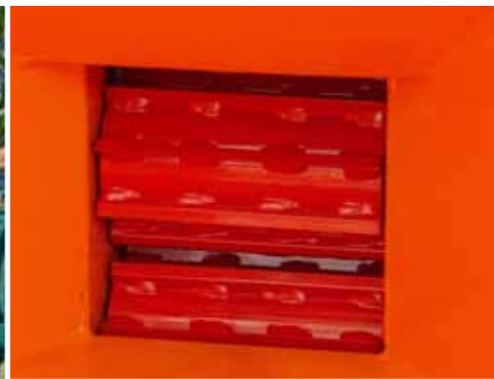
Rollers conveying the material to the set of shredding knives.
