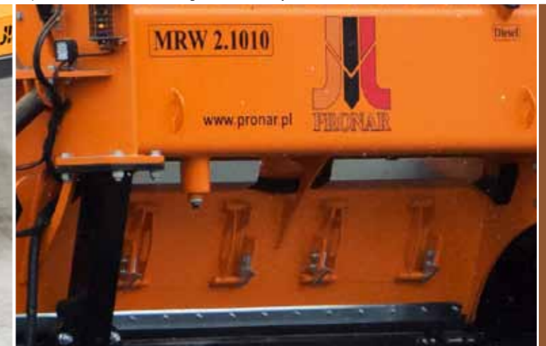
Inspection windows of the working chamber for easy cleanout and maintenance
