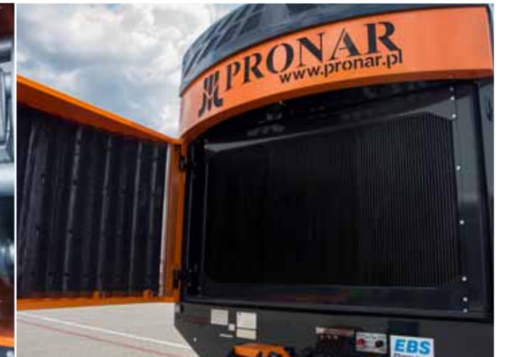
Reversible radiator Keeps engine and hydraulic oil coolers clean in dusty environment.
