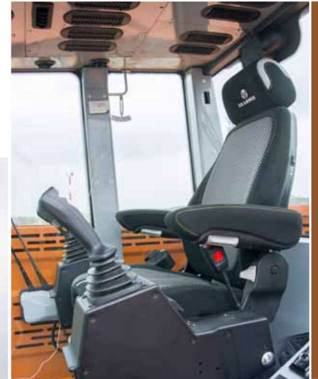
An ergonomic pneumatic suspension seat with automatic positioning, weight control, vibration damping has been installed in the cab
