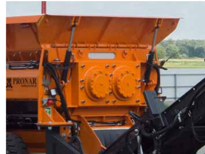
Easy to remove cassette with shafts significantly shortens time for switching machine for work with different material.
