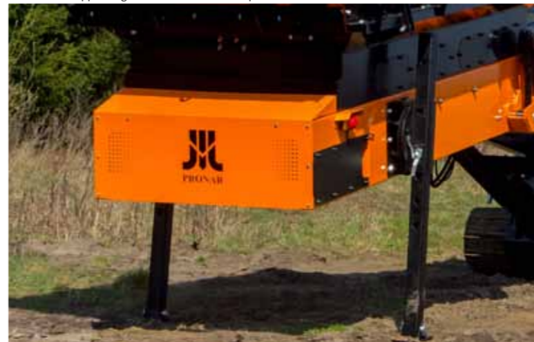
Mechanical support legs at the rear of the stockpiler
