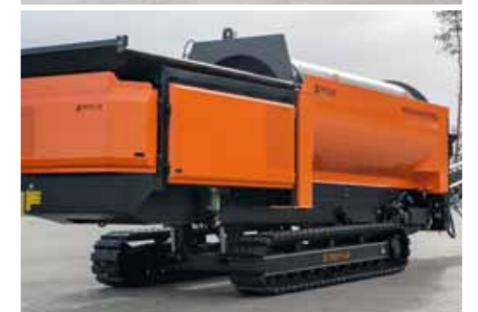
Hydraulic system for adjusting chassis position in MPB 20.55gh. The mechanism allows leveling machine on longitudinal slopes and increases the clearance for easier moving on uneven terrain
