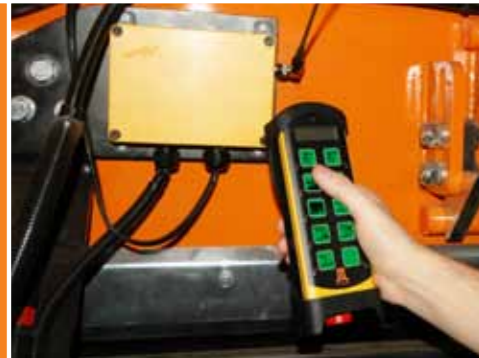
Remote control for basic machine operating functions
