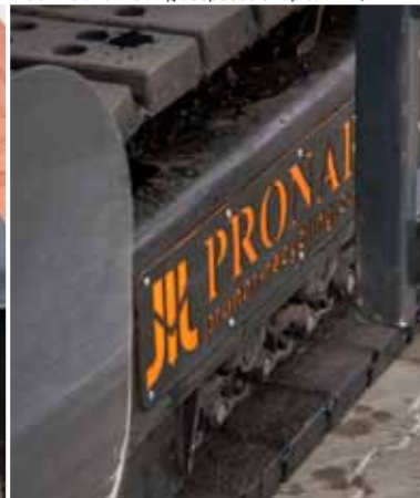
Track drive allows convenient maneuvering of the machine and moving at speeds of up to 4km/h
