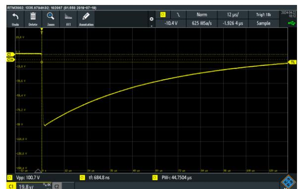
**Negative Dry Lightning Impulse Oscilloscope Graphics**
