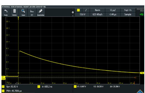
**Positive Dry Lightning Impulse Oscilloscope Graphics**
