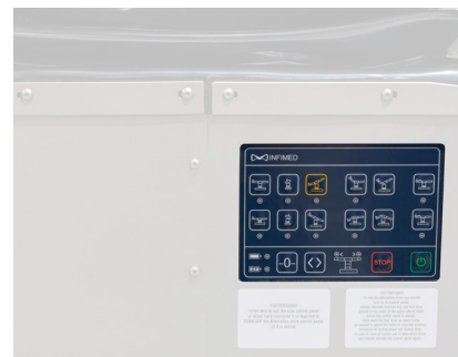
Sensor side control panel
