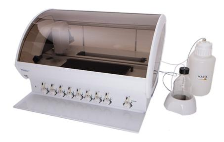
The Dynablot Automatic is a fully automated instrument for LINE Immunoblot testing. The LabImage® LA software is used for result interpretation and evaluation.
