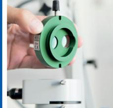
**Removing the protection filter from a slit lamp
