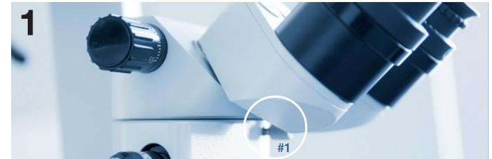
2) Open the screw #1 to remove the ocular. Insert the protection filter according to the image (3)
